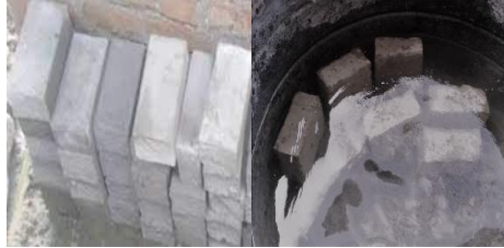
Fig 2. Concrete bricks in water for Water absorption Source: Self
