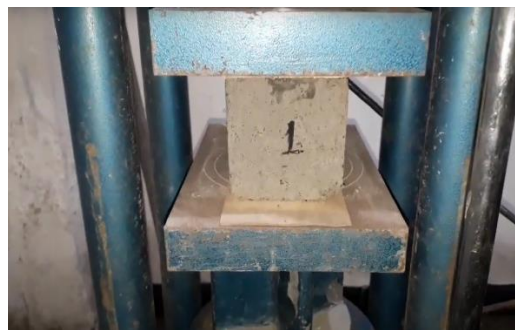
Fig 1. Compressive test machine (Source: Self)
